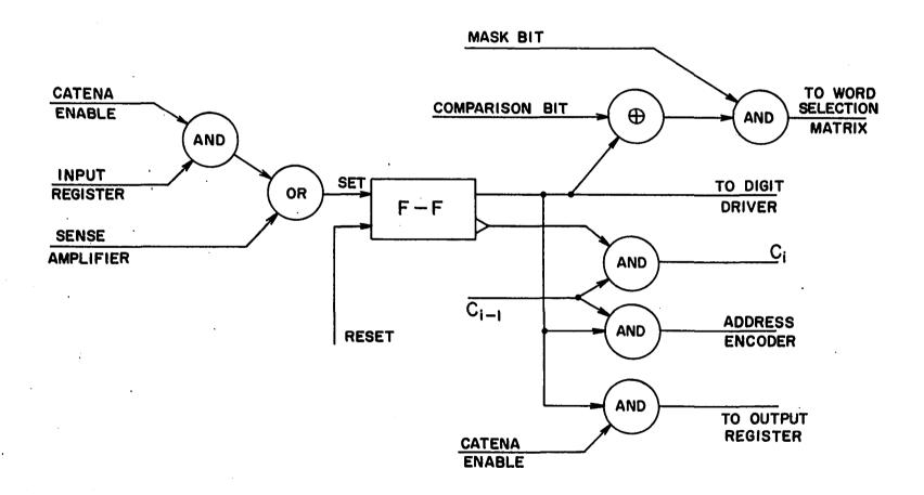
Fig. 17. Circuitry required per catena bit
