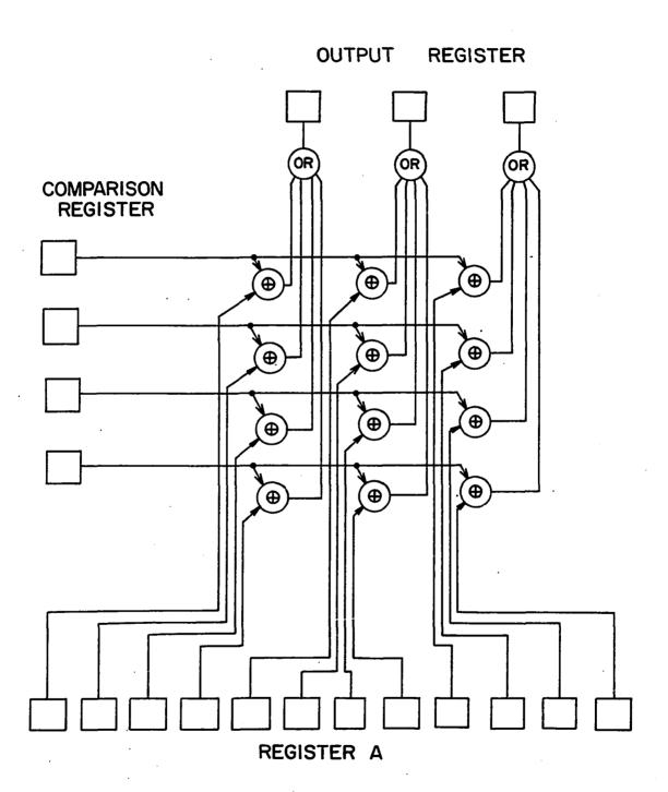
Fig. 16. Output logic required per bit
